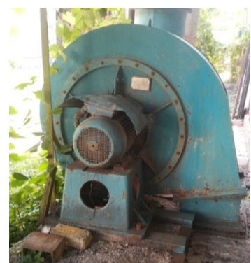
The system of air supply to the burner
